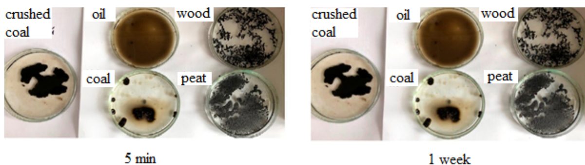
Fig. 2. Kinetics of removing engine oil film by adsorbents from secondary raw materials
